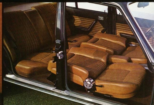
When we say fully reclined seats...we mean flat out! Retractable headrests make this possible. Front seats slide back and forth on curved rails (ball bearings, spring return), automatically adjusting to the height of all size drivers.
